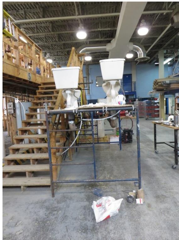
Figure 4-3 : Toilettes et raccordement
